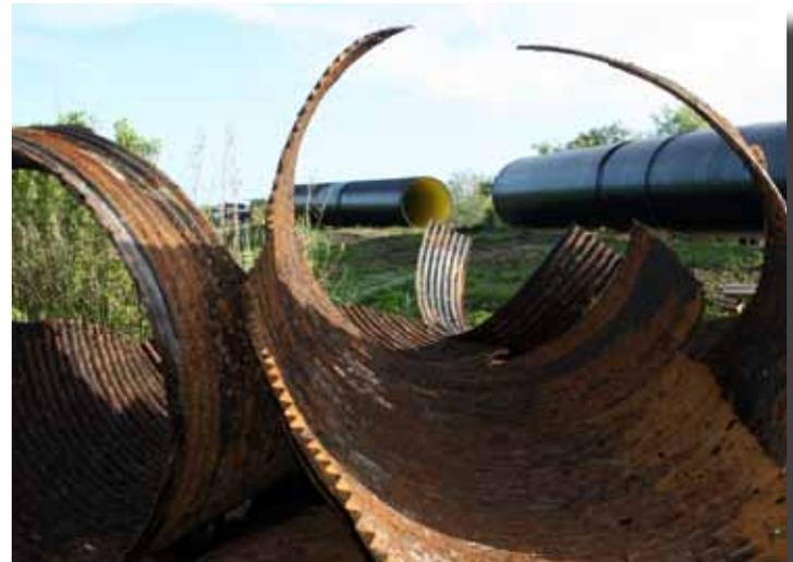
*A view of the excavated deteriorated corrugated metal pipes with the new profile wall pipe liner in the background.*
